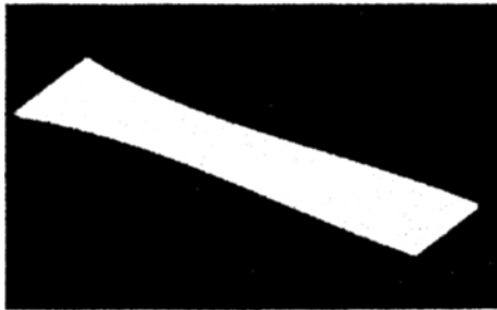
Fig. 10 Beam shape which maximizes fundamental natural frequency
